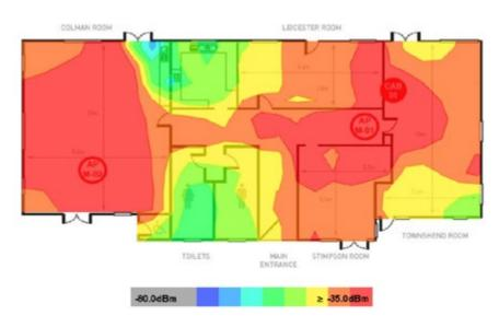
This provided physical access point locations, detailed information on the mounting of the access points as well as annotated photos. The required cable runs for each and the relevant health and safety information for completing their installation, which was later provided in a Risk Assessment and Method Statement. 2.4 GHz & 5 GHz heatmaps of the prospective coverage and all-important
